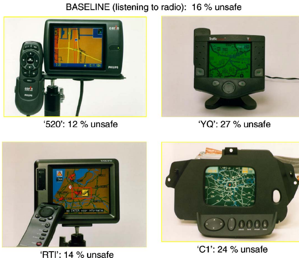
Fig. 1. Percentage of a set of manoeuvres performed in an unsafe way for different commercially available RDS-TMC systems (Janssen et al., 1999).
